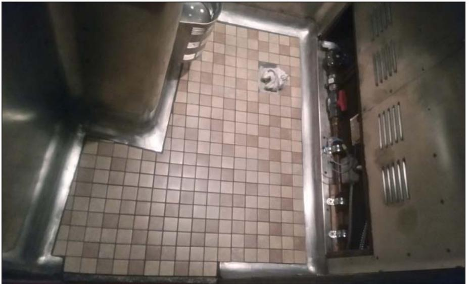
the window band, the bathroom lounge, the end walls of the seating area, and the locker and closet doors have been sanded and filler applied where necessary. After a few more touch-ups, we will use matching tan interior paint to get the car looking good inside. Once the interior paint is set, the floor can be stripped and waxed and the seat frames and upholstery reinstalled.
